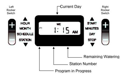
During an AUTOMATIC watering cycle, stations (zones) may be advanced by momentarily pressing RIGHT ROCKER SWITCH as START. Water cycle will continue from the indexed station to the last station programmed with a watering duration.
